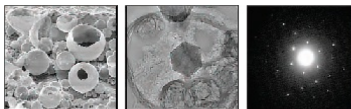
Figure 4.11: Protein-encapsulated water. Encapsulation produces spheres (a) seen in the scanning electron microscope, and geometric figures (b) seen in the transmission electron microscope. Diffraction pattern (c) obtained from a geometric figure shows hexagonal order.
